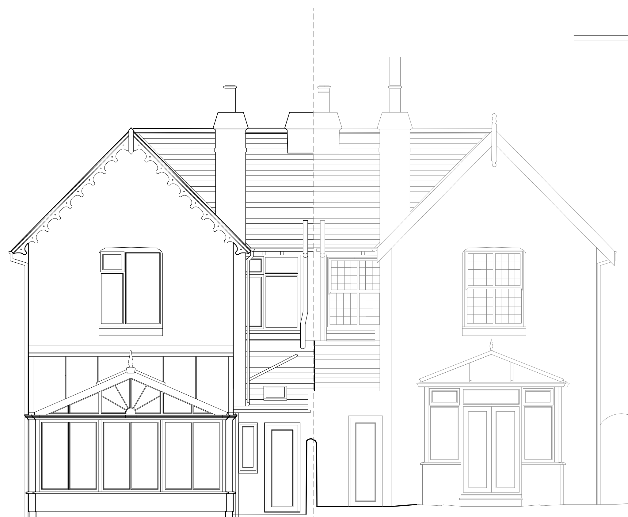
REAR ELEVATION 1:50 (Showing proposed neighbours extension)
